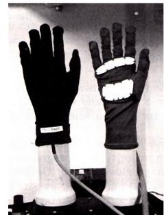
Abb. 46 ADVANCED ROBOTICS RESEARCH CENTER TELETACT I TACTILE FEEDBACK GLOVE [QB02]
